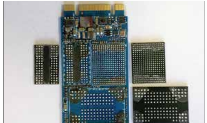
Fig. 12: Underfilled components after desoldering
