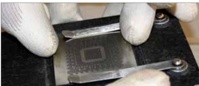
Fig. 16: Reballing module, template is aligned
