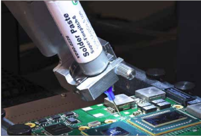
Fig. 18: Dispensing of solder paste
