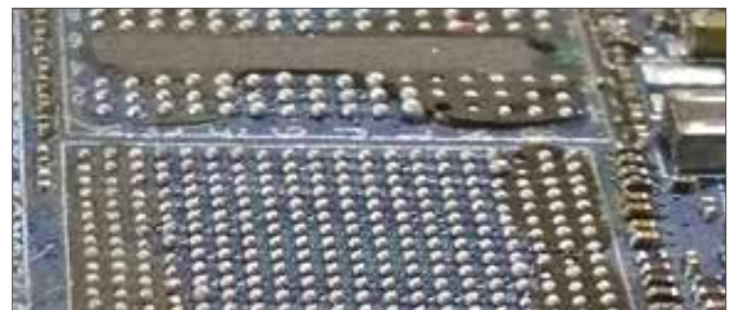
Fig. 13: Underfill residues after component removal
